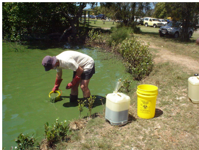
Figure 1 Field collection of bloom material for cyanotoxin extraction. Unobtrusive and common-sense personal protective equipment - waterproof boots and gloves in this case - may be used to harvest bloom biomass. Workers undertaking such activities should be familiar with the risks of accidental immersion, however, and care must be taken to ensure a secure footing. Photo by author WAW.
