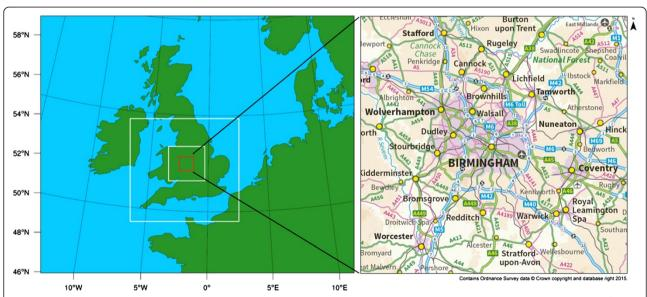
**Fig. 1** Geographic area covered by the WRF model simulations. Model resolution increases as boxed domains decrease in size, and is 1 km<sup>2</sup> in the central domain (red box) which covers the West Midlands region study domain (right), which is approximately 81 km by 78 km
